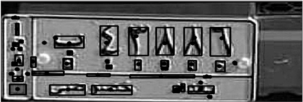
Figure 19. Arabic license plate connected component analysis result, showing the dot component of the (ب) letter being detected as a separate entity
